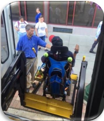
Centro Call-A-Bus vehicles are equipped with a lift to accommodate wheelchairs. Some oversized wheelchairs may exceed the lift capacity and cannot be accommodated. If you have concerns about your wheelchair's size or weight fitting on our vehicles, please contact your local Call-A-Bus office and we will make arrangements to have a supervisor inspect your wheelchair.
